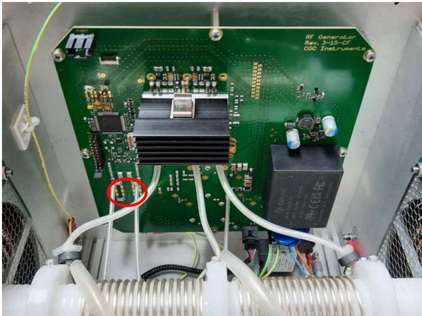
Fig. 4. View of the generator's printed circuit board. The red circle marks the capacitors Co1 and Co2 for adjusting the resonance frequency of the output circuit.
