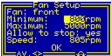
Fig. 5. Setting the rotational speed of the particular fan in the dialog box "Fan Setup".
