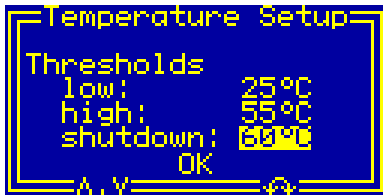
Fig. 9. Setting the shutdown temperature in the dialog box "Temperature Setup".
