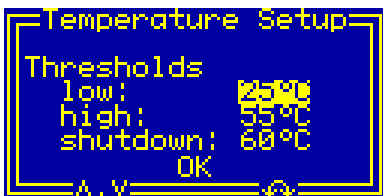
Fig. 8. Setting the low temperature threshold in the dialog box "Temperature Setup".
