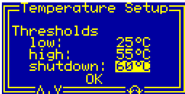
Fig. 9. Setting the shutdown temperature in the dialog box "Temperature Setup".
