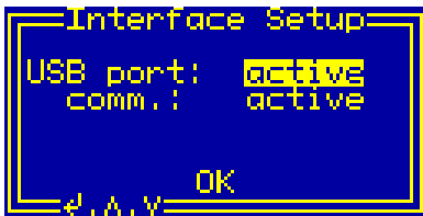
Fig. 11. Enabling the USB interface in the dialog box "Interface Setup".
