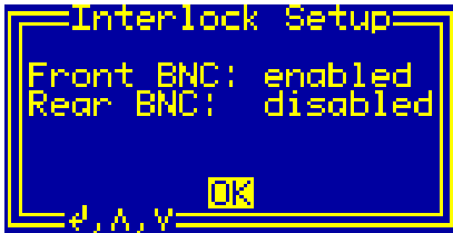
Fig. 9. Setting the interlock function in the dialog box "Interlock Setup".
