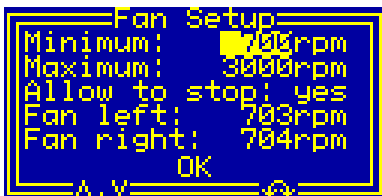
Fig. 36. Setting the rotational speed of the fans in the dialog box "Fan Setup".
