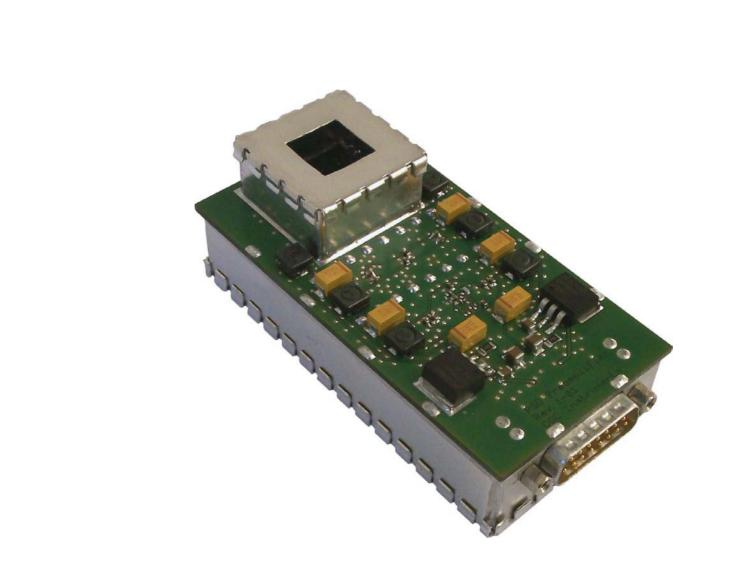
PSD (Position-Sensitive Detector): measures the microparticle's position DCD (Coordinate-Decoder Unit): obtains the coordinate signals
